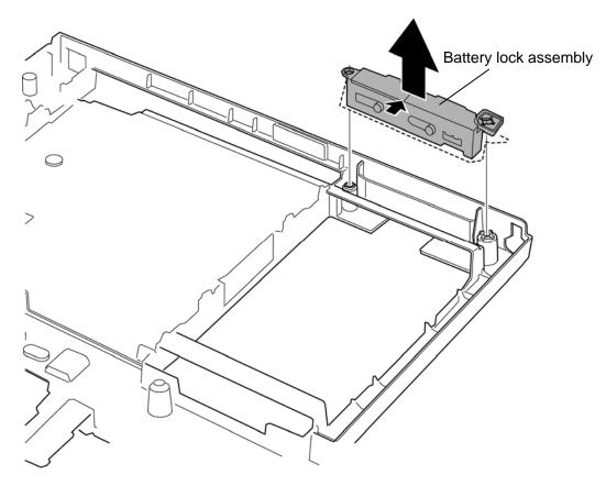
Figure 4-27 Removing the battery lock assembly
